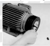
Place lubrication oil on blot Screw one of the bolts into a removal hole until bushing comes out about 5mm. If removing the bolt is difficult, hit on the hub of the sheave with a hammer.
