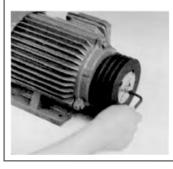
Fasten with wrench (torque wrench is better if bolt is tough to screw on). Lightly hit on hub of sheave with a hammer screw gradually and alternatively give a little grease into a removal hole.
