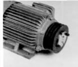
Bushing should not be fastened to final positions. Bolts screwed-up about two thirds of the overall length.
