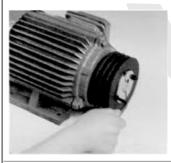
Bushing is still loosely fastened Expand the bolt with the screwdriver to insert easily. Loosen taper-fitted bushing from shaft.
