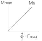
M<sub>max</sub>--Required transmitted torque Nm F<sub>max</sub>--Required transmitted axial force N Mh--synthetic transmitted torque Nm d--Transmission shaft diameter mm Mt--NSPT LOCK rated transmitted torque Nm
