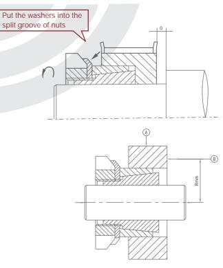
After the correct installation mentioned above inspect the runout for (A) and (B). The run out for (A) should not excess 0.05mm and 0.02mm for (B).
